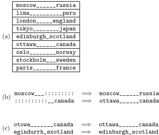
Figure 44.2. Associative memory (schematic). (a) A list of desired memories. (b) The first function of an associative memory is pattern completion, given a partial pattern. (c) The second function of a memory is error correction.
