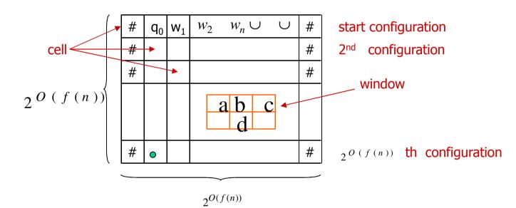
The content of d is determined by the contents of its parents a, b, and c.
