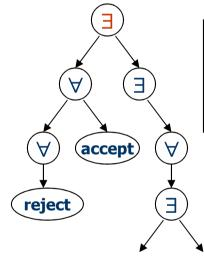
An ATM is an NTM with all states, except accept and reject states, divided into universal states and existential states.
