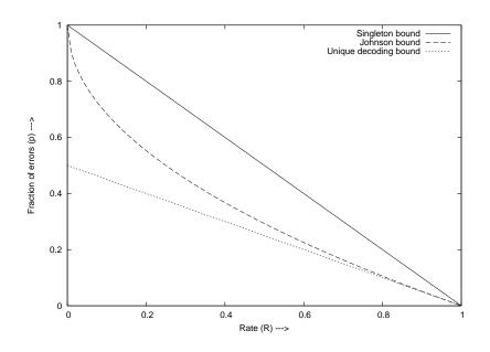
Figure 1: The tradeoff between rate R and the fraction of errors that can be corrected.  $1 - \sqrt{R}$  is the tradeoff implied by the Johnson bound. The bound for unique decoding is (1 - R)/2 while 1 - R is the Singleton bound (and the list decoding capacity for codes over large alphabets).
